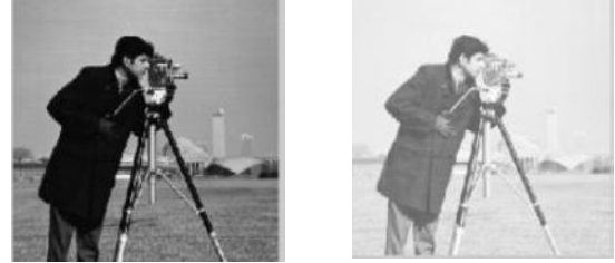
Fig. 4: Original Image and its Logarithmic Image
