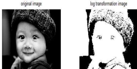
Fig. 2: Image Enhancement Using Image Log Transform
