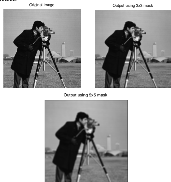
Fig. 5: The Original Image and Output using 3x3 Mask and 5x5 Mask
