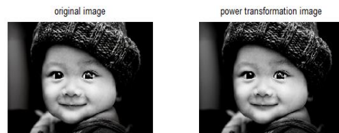
Fig. 5: Image Enhancement using Power Law Transform
